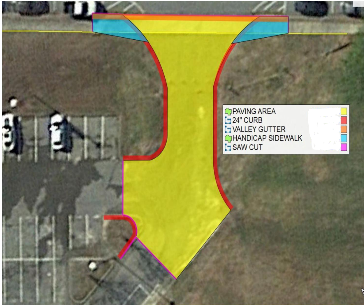
DHS West parking lot: Existing construction entrance to school.
